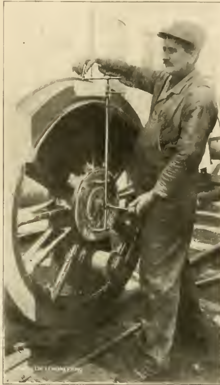
DRIVING WHEEL TIRE CALIPER USED IN THE OSWEGO SHOPS OF THE R. W. & O.
